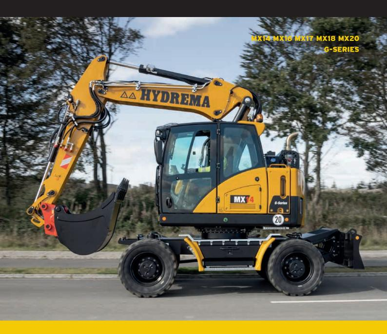
Efficient, powerful and stable wheeled city excavator. Excellent lifting capacity and very compact dimensions.
